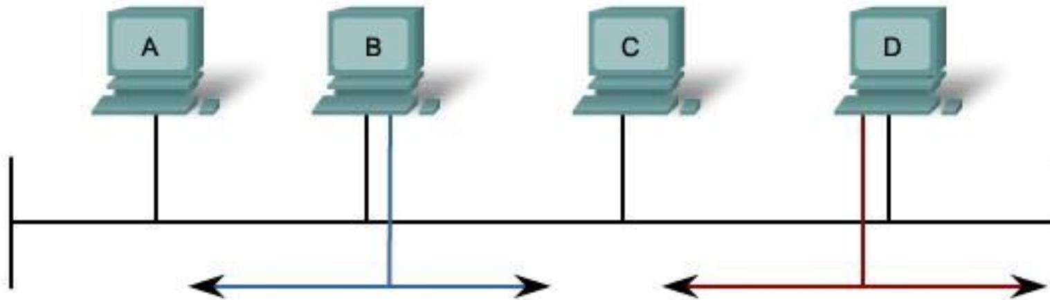
CSMA/CD controls access to the shared media. If there is a collision, it is detected and frames are retransmitted.
