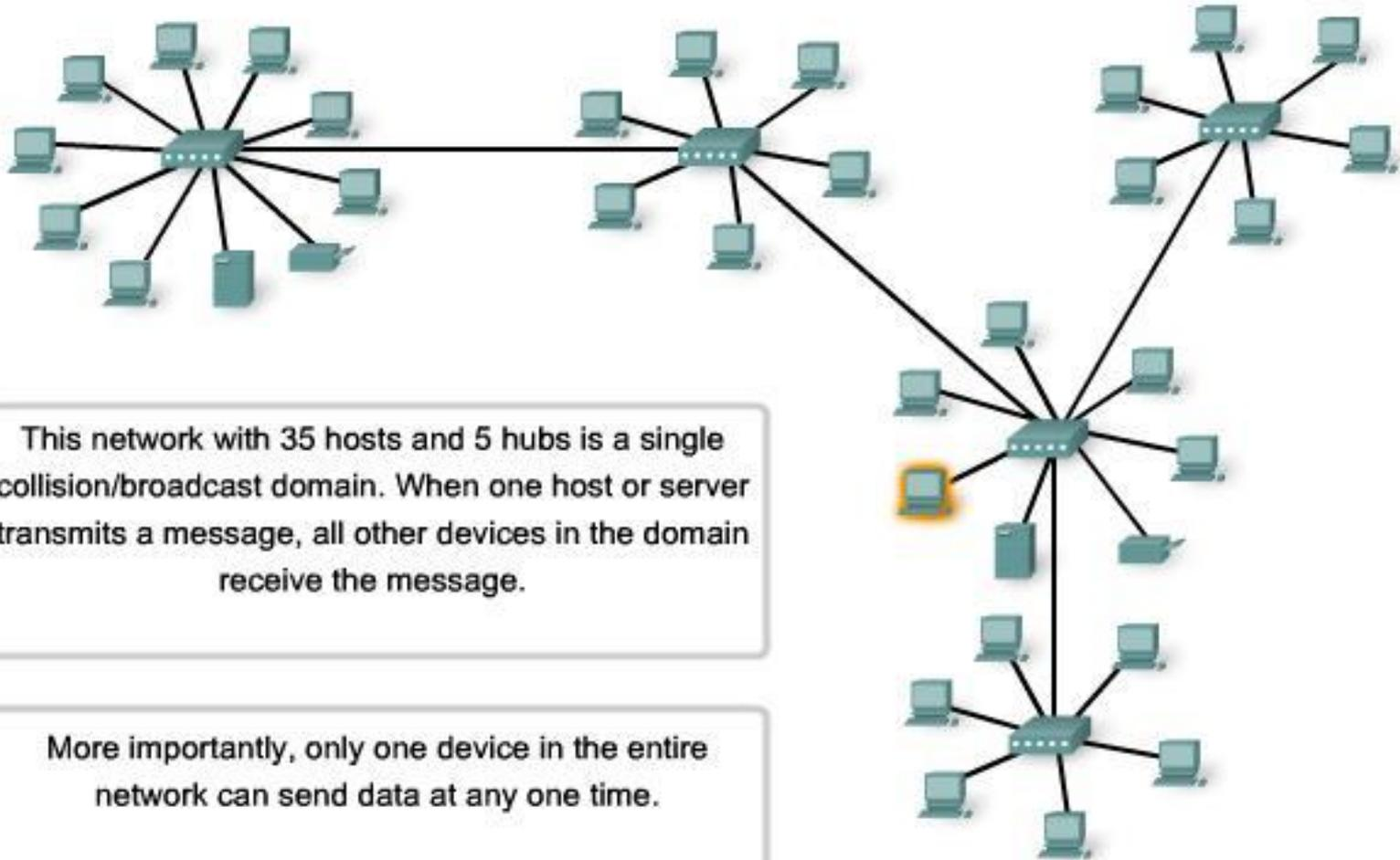
This network with 35 hosts and 5 hubs is a single collision/broadcast domain. When one host or server transmits a message, all other devices in the domain receive the message.
