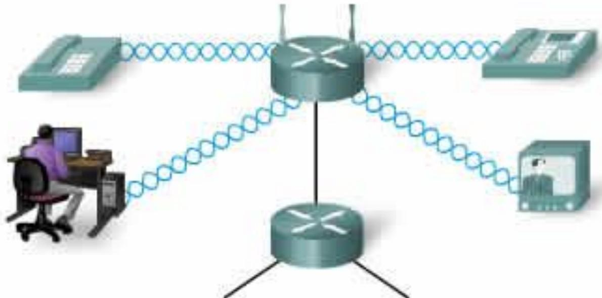
Wireless networks are also connected to wired networks, at some point.
