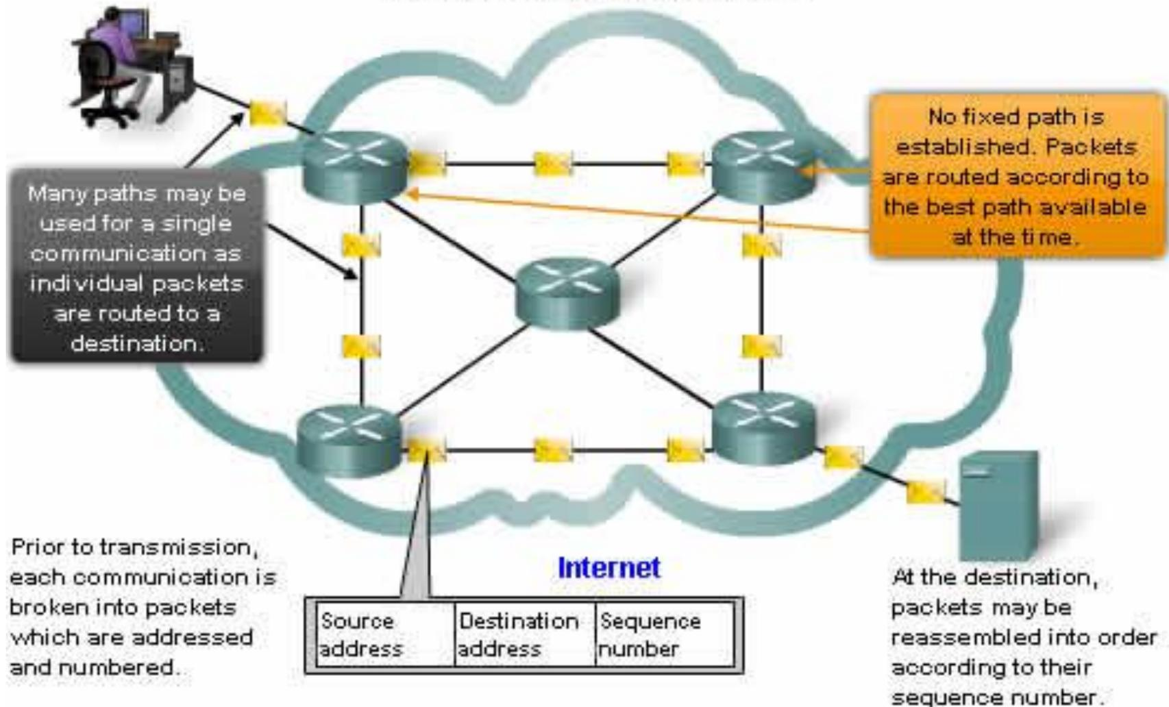
Prior to transmission, each communication is broken into packets which are addressed and numbered.
